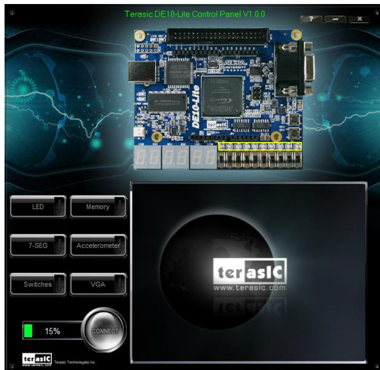
Figure 2-1 The DE10-Lite Control Panel
