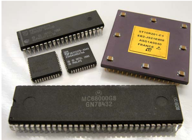
Figure 9: Original MC68000 8 MHz (current M68K chips are the same size as the original die of this part) ST10R201 bond-out from STMicroelectronics (16 bit), 44 pin S87C51FB from Philips (now NXP) 40 pin Philips 8051, 44 pin 80251 - 16 bit 8051. Chips today are much smaller than these. The big 8051 is 2 inches long, small chips are almost ¾ inch and the 68000 is 3 ¼ inches and has 64 pins.
