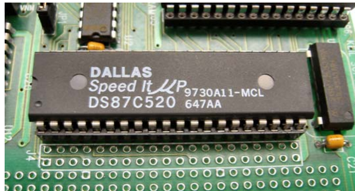
Figure 5: Dallas Semiconductor was one of the first companies to offer reduced cycle per instruction parts. We can assume this part was made in the 30 th week in 1997. (9730)
