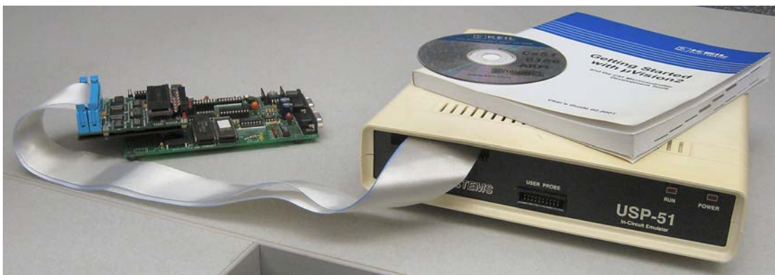
Figure 4: Signum Systems In-Circuit Emulator with OKI probe debugging the Keil 8051 board. Few people work with these anymore: but this technology was vital for the development of the 8051 market. You can still buy these products but both Keil and Signum (and others) also offer solutions for today's 8051.
