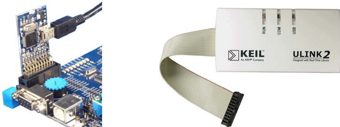
Figure 10: USB to JTAG Adapters: ULINK-ME (left) and ULINK2 (right). They work with JTAG, Infineon OCDS and FS 2 as found in NXP processors and are quite flexible. The ULINK2 can connect to various target connector standards.
