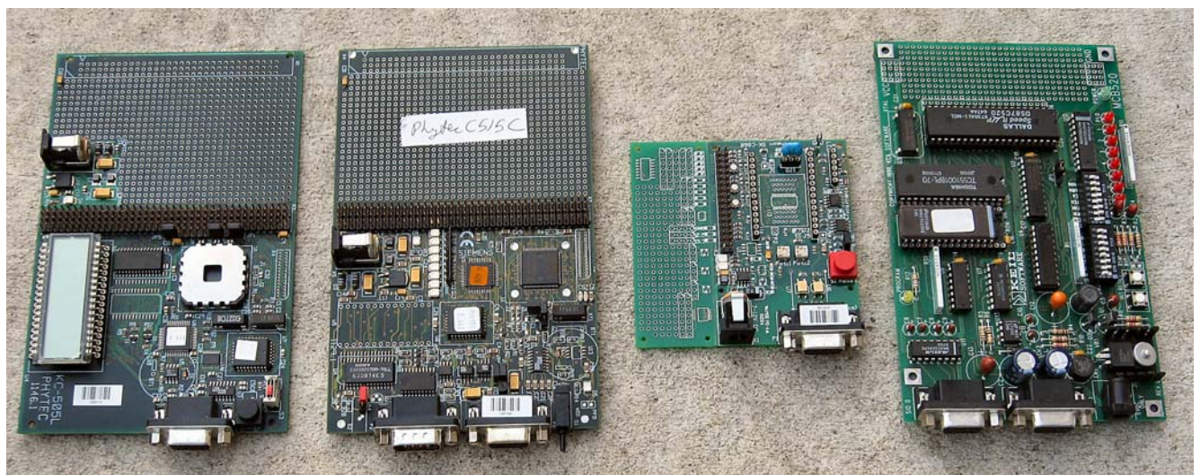
Figure 7: 8051 evaluation boards: – Phytec C505L, C515C, C868 (all Infineon) and Keil 8051
