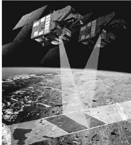
Figure 10.33 High resolution stereoscopic (HRS) instrument (Reproduced by permission of Spot Image - © CNES)
