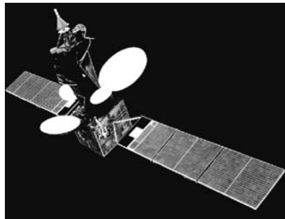
Figure 3.31 Three-axis stabilized satellite (Intelsat-5) (Reproduced by permission of © Intelsat)
