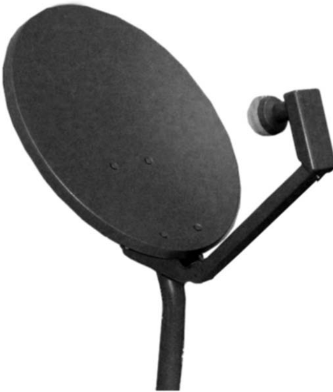
Figure 8.27 DTH dish and co-located LNB
